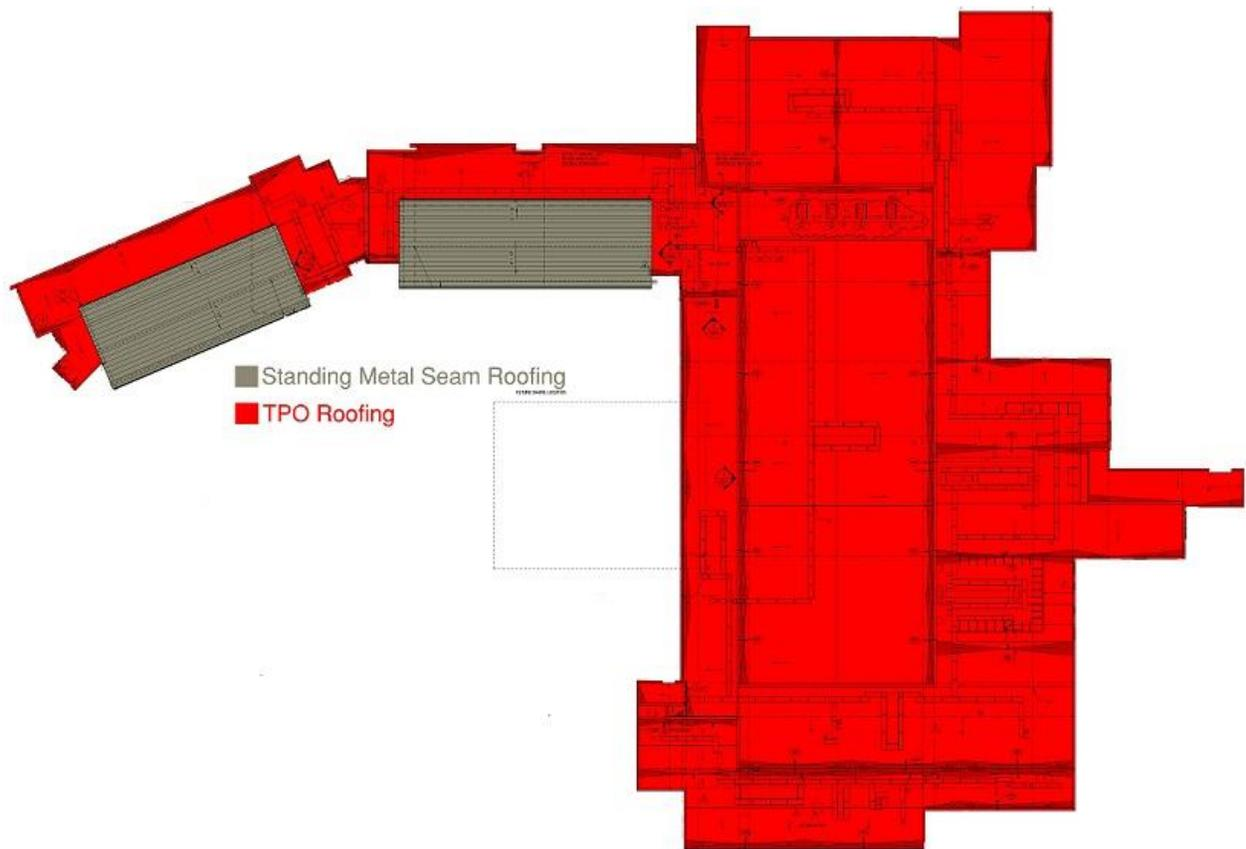
The addition of a photovoltaic system has left me with a huge opportunity to conduct an Electrical Breadth on this topic. It must be determined how the system loads will tie together and how it will aid in the load reduction of the building, as well as any equipment sizing reductions. Shown below is a roof plan displaying the different roofing systems. The standing seam system is shown in gray and the TPO system is shown in red:
